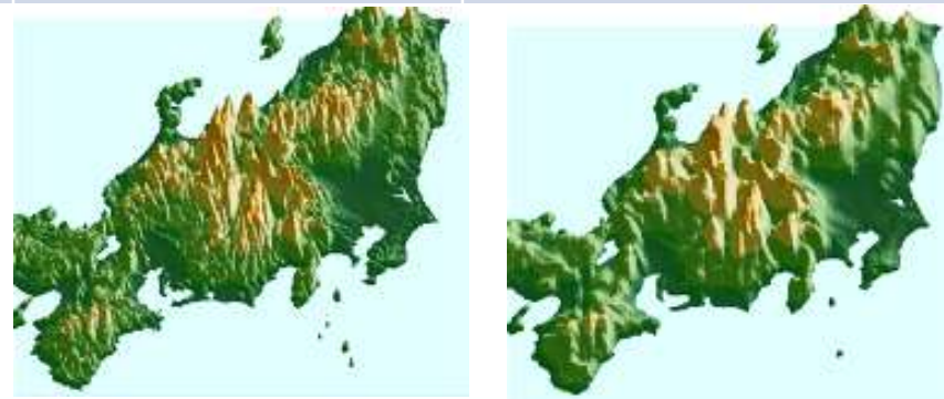
Terrain of the central region of the Main Island of Japan used for the LFM (left, 2-km horizontal resolution) and for the MSM (right, 5-km horizontal resolution)
